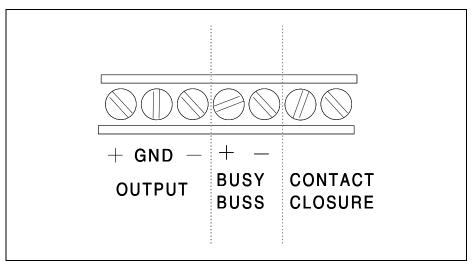
Figure 3. Wiring Connections on Microphone Terminal Block
